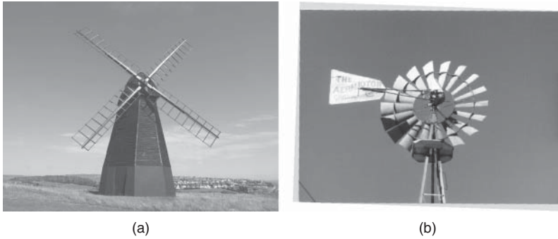
Figure 1.4 A traditional windmill (a) and an American farm windmill (b) for pumping water.
